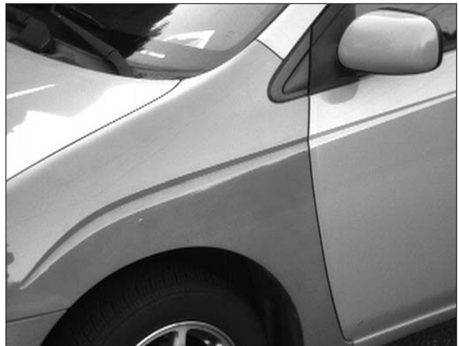
Figure 5a and Figure 5b —Here is another example of what can be found with longwave UV procedures. The car shown above has had its driver's side front fender replaced. Under longwave UV imaging (Figure 5b), the difference is obvious. (Photos courtesy of Austin Richards)
