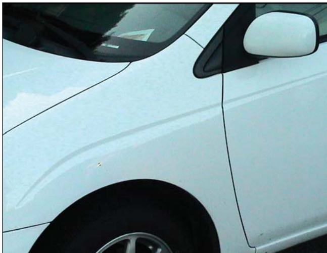
Figure 5a and Figure 5b —Here is another example of what can be found with longwave UV procedures. The car shown above has had its driver's side front fender replaced. Under longwave UV imaging (Figure 5b), the difference is obvious. (Photos courtesy of Austin Richards)
